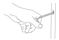
4. Tighten the frame adjusters clockwise, with a 5mm ball-ended Allen key, until the ends of the spreader plates are flat against the wall.
