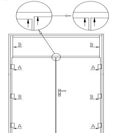
3. Align and grip the doorset in the opening, using the frame adjusting screws A in the corners, then the middle adjusters B.
