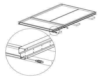
2. Slide transom between jambs then attach to frame with taptite screws. Tighten all screws.
