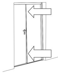
7. Open the doors, discard the transit packings, then close and lock the fixed leaf. With the active leaf nearly closed, check the alignment between the active leaf lock edge, and the slam bar frame seal, at both the top and bottom of the doors.
